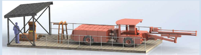
The semistatic pull-brake tester avoids damaging the brake system and is a safe means of testing the surface, neutral and park/emergency brakes.
